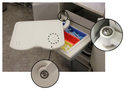
Swing-out shelves include two simple tension adjustment points—one on each side of the shelf arm (one above and one below the shelf). Use a 5/16" hex key to adjust the tension.
