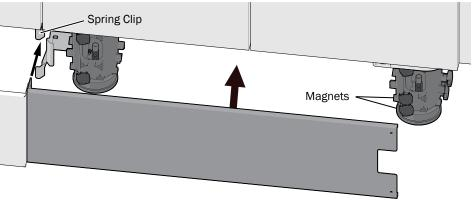
Cabinet base covers are easily removed for cleaning or to access utilities. Pull the covers straight out to remove them. When you reinstall the covers, make sure they attach in their original location onto magnets or inserted into spring clips. Place the rounded corner base covers on the front corners of the cabinet and the square covers on the back corners.
