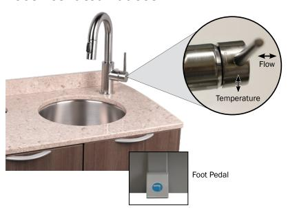
For sink modules that include a foot-activated faucet, water temperature and flow are determined by the faucet handle position. To set, press the foot pedal and move the faucet handle until you reach your desired temperature and flow rate.
