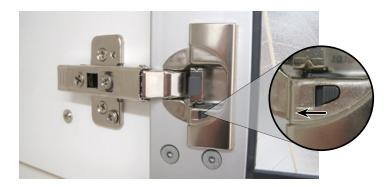
You can deactivate the soft-close feature, if desired. To deactivate, slide the black switch toward the cabinet on all hinges for that door.
