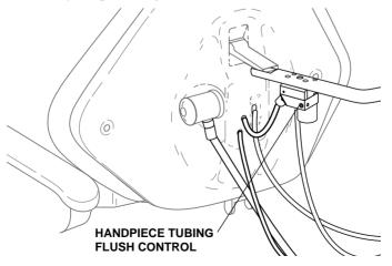
Figure 6. Handpiece Tubing Flush
