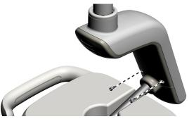
**2** Use two screws to secure the cover.
