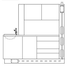
1 Route the conduit to the junction box below the sink module.
