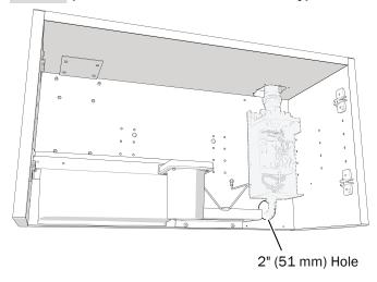
**1** Drill a 2" (51 mm) hole in the cabinet and wall about 2" (51 mm) below where the power supply will be mounted. The hole is used for routing the conduit and data line.
