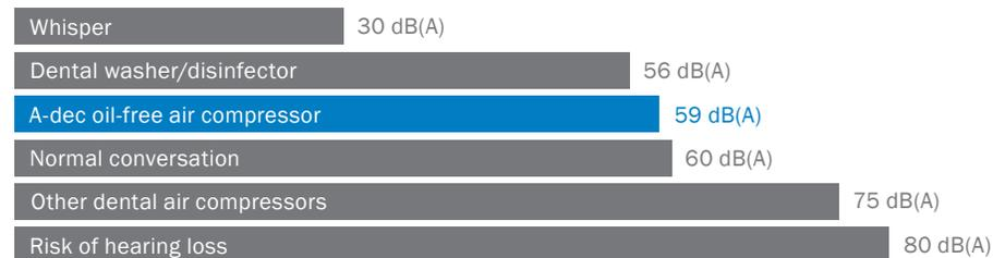
Source: National Center for Environmental Health. Dental washer/disinfector dB(A) and average dB(A) for other air compressors based on manufacturers' specifications.
