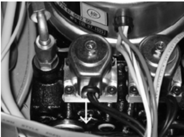
Figure 4. New solenoid inserted with the wire facing away from the pump.
