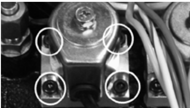
Figure 2. Removing the socket head screws from the solenoid.
