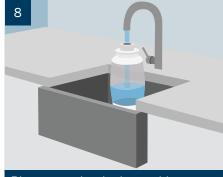
Rinse water bottle thoroughly. Refill bottle with water and flush through DUWL until empty.
