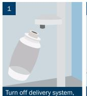
Turn off delivery system, remove and empty the water bottle.
